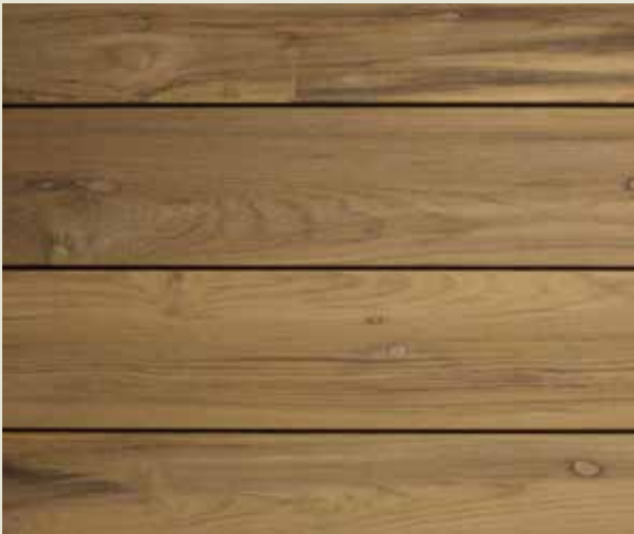
WOOD FOUND ON BENCHES AND EDUCATION BUILDING - TEAK Species: Tectona grandis Certification: FSC Recycled 100% - FSC-C021798
